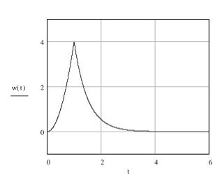
Energy is being stored in the capacitor whenever the power is positive. Hence energy is being stored in the interval 0 to 1 s.
