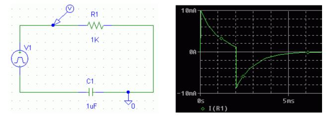
So now, we are ready to measure the output signal. We change the place of the ground and get the response of the circuit to this input signal.
