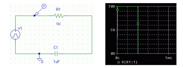
This is our circuit in PSpice. At first, we measure the input signal by putting the ground next to impulse generator. The input signal is seen on the right side.
