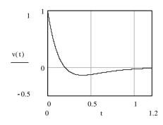
e) If we notice, we see that at t=0.2 s the voltage changes polarity. This is the instant when current is maximum.
