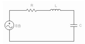
In the RLC circuit in the figure above, the voltage drops across the inductor, resistor, and capacitor are given by  $L\frac{di}{dt}$ , Ri, and  $\frac{1}{C}\int\limits_{0}^{t}i(\tau)d\tau$
